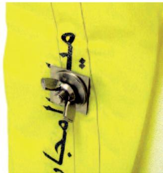
Wavelay<sup>®</sup> clamped to an access chamber wall makes direct connection by a cable & pipe locator / detector easy.
